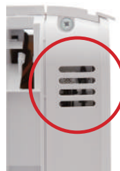
Sensor for indoor temperature and humidity
